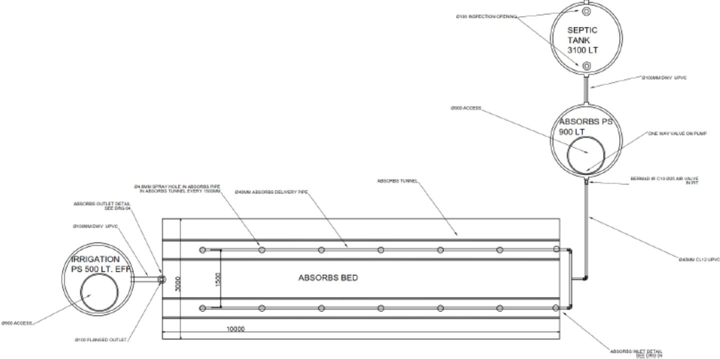
Figure 2 Typical ABSORBS™ system layout (lined configuration)
