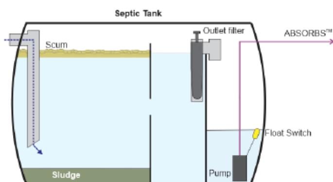
Figure 3 Schematic of your pre-treatment system
