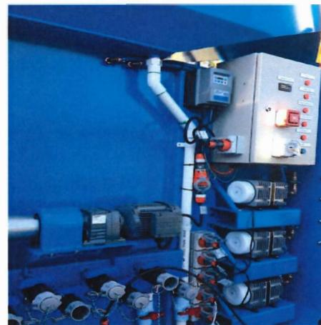
Individual Air Pumps operate in each tank, providing regulated air through the Dissolved Oxygen Metre. The Oxygen metre is heat compensated
