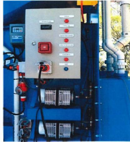
PLC—Programmable Logic Controller fully automates the unit for easy operation. Audible alarms are in place to manage malfunctions with troubleshooting backup
