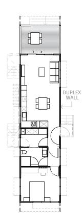
ALTERNATIVE FLOOR PLAN Linear Arrangement SCALE 1:200 at A4
