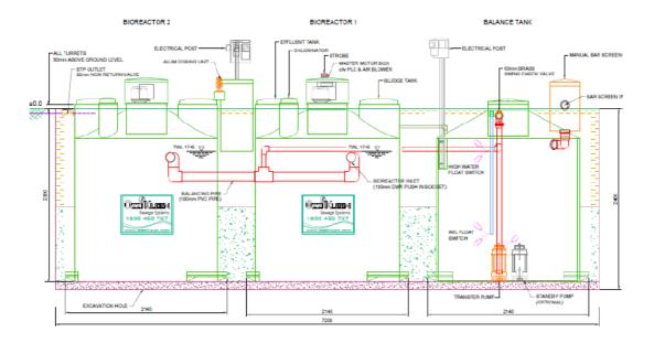
Figure 2. RP20A Below Ground Treatment Plant
