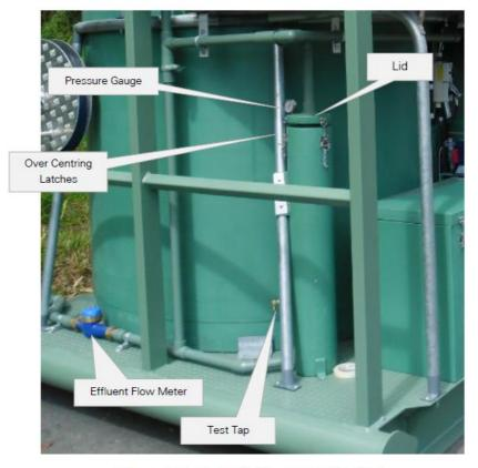
Photo 2. Sock Filter and Effluent Outlet Pipe Work
