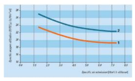
Oxygen utilization in clean water, ELASTOX®-T type B
