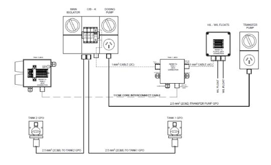
Figure 4. Electrical Connections Required at Installation
