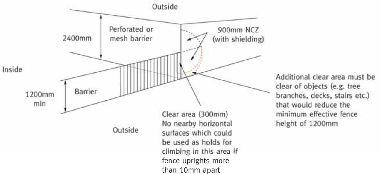
Note: The non-climbable zone (NCZ) continues in spherical form at the intersection of the pool barrier with the structure to the wall of the structure. The additional clear area continues in an arc past the intersection to the wall of the structure.
