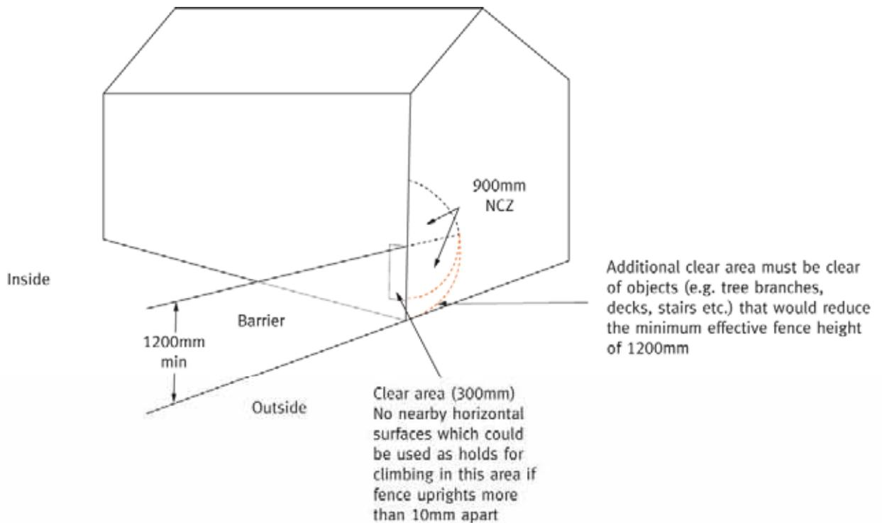
Note: The non-climbable zone (NCZ) continues in spherical form at the intersection of the pool barrier with the structure to the wall of the structure. The additional clear area continues in an arc past the intersection to the wall of the structure.
