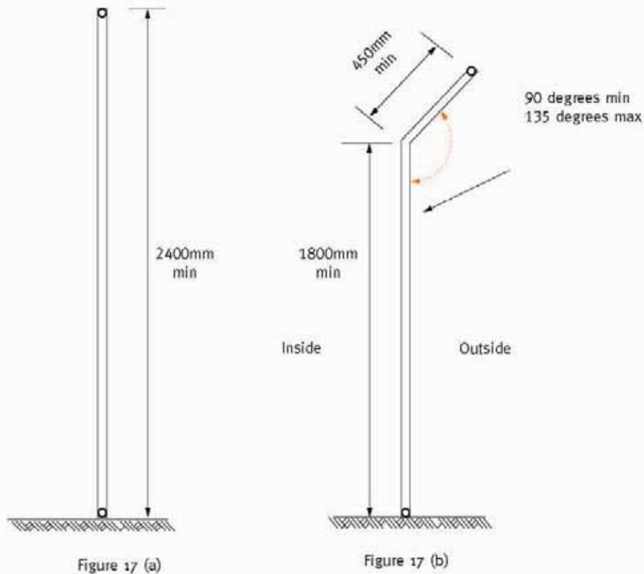
Note: Barriers using perforated material or mesh with apertures greater than 13mm but less than 100mm shall comply Figure 17(a) or (b) Barriers using mesh must include a strainer wire or rail at the top and bottom of the fencing In Figure 17(b) the cranked top shall have apertures less than 100mm
