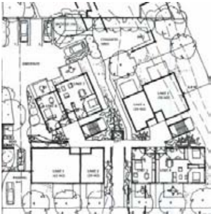
Lot 10 at KGUV ensures that cross ventilation of units is achieved through breezeways.
